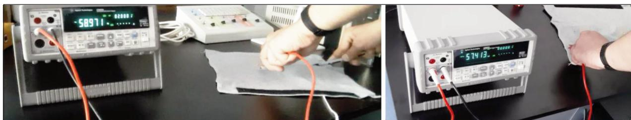
Fig. 2. Determination of the variation of the electric current in the conductive textile electrodes and of the frequency
